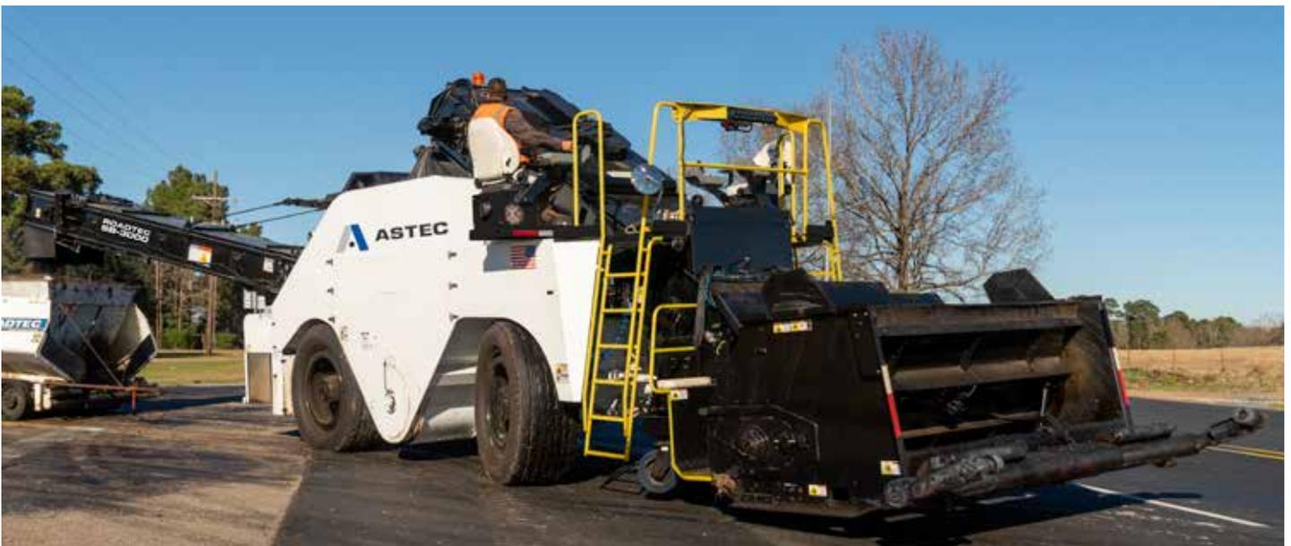
*The dump truck is not able to maneuver into the intersection of this jobsite. The SB-3000 solves this problem. The mix is dumped from the dump truck into the SB-3000's hopper and shuttled to the intersection where it is placed into the waiting paver.*
