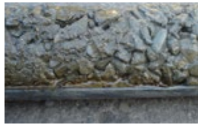
Contaminated sand with gravel. Sampled with AquaLock 70
