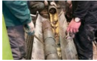
Permafrost, sand and gravel. Sampled with CB8 SingleWall Core barrel
