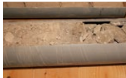
Railway sample 180mm. Sampled with CB 8" Single Wall Core Barrel
