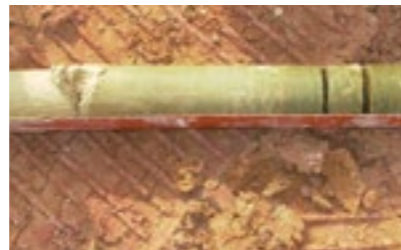
Hard consolidated clay going over in very soft clay. Sampled with CB4" Single Wall Core Barrel
