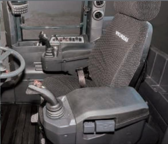
The HL970A has a **large, comfortable, air suspended seat** with heating as standard. The seat and armrest are fully adjustable.
