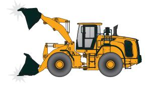
The **soft end stop** function reduces the hydraulic speed of the cylinder as it reaches the end of its stroke. This lessens the shock load of the stroke for increased operating comfort and better material retention.
