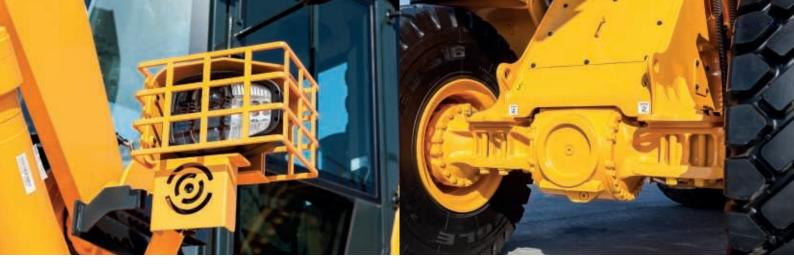
A steel grill housing protects the front and rear working lights from material spill from the bucket.
