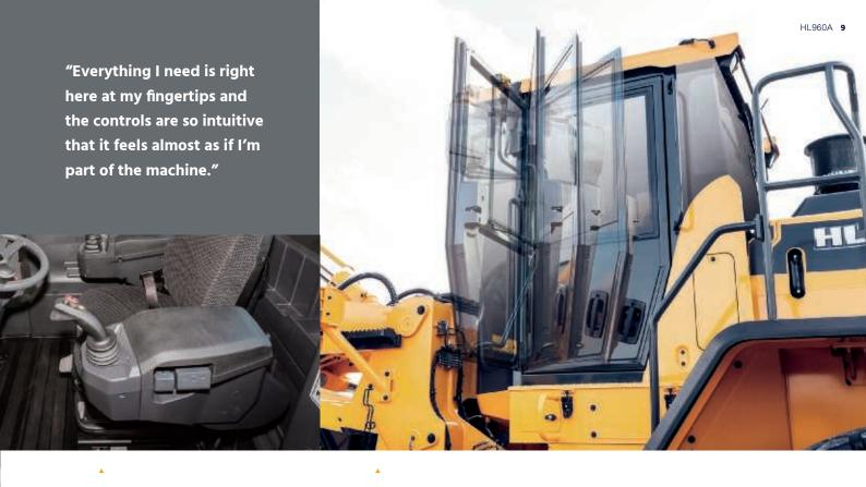
The HL960A has a large comfortable seat with heating as standard. The seat and armrest are fully adjustable and, for added comfort, an air suspension version is available as an option. Thanks to the **electro-hydraulic implement control lever**, less force is needed to operate attachments, helping you to work longer and more productively.
