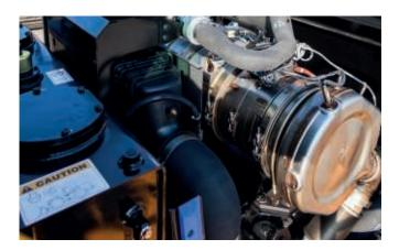
Like all A-Series machines, the HL 960A features our all-inone exhaust aftertreatment system which cuts emissions and operating costs while enhancing reliability and simplifying maintenance.
