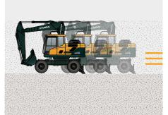
cruise control and speed limiter systems, allowing operators to relax while maintaining a steady speed over longer distances. When creep speed is activated, the excavator will drive at a maximum speed of 3.5 km/hr. This gives the operator better control and higher torque with minimal effort.
